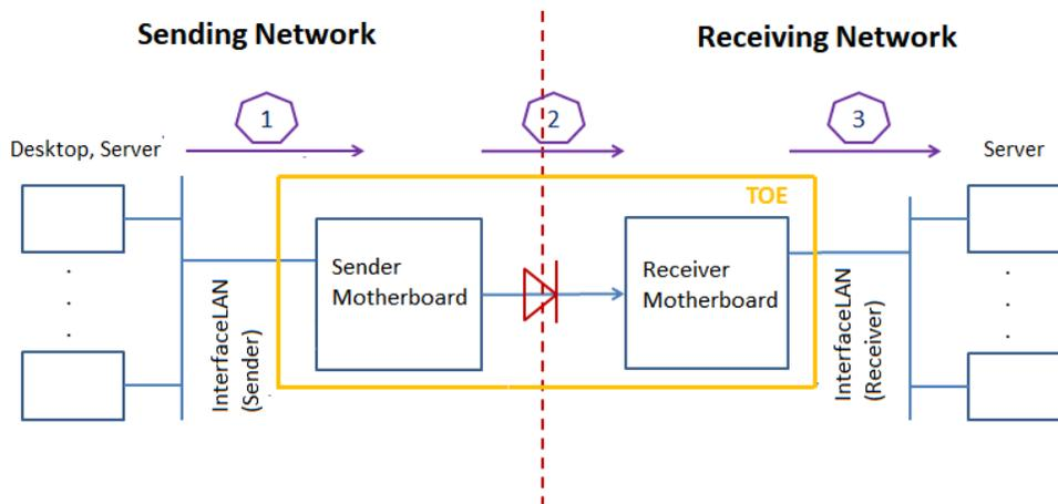
**Figure 3: TOE Data Flow**
