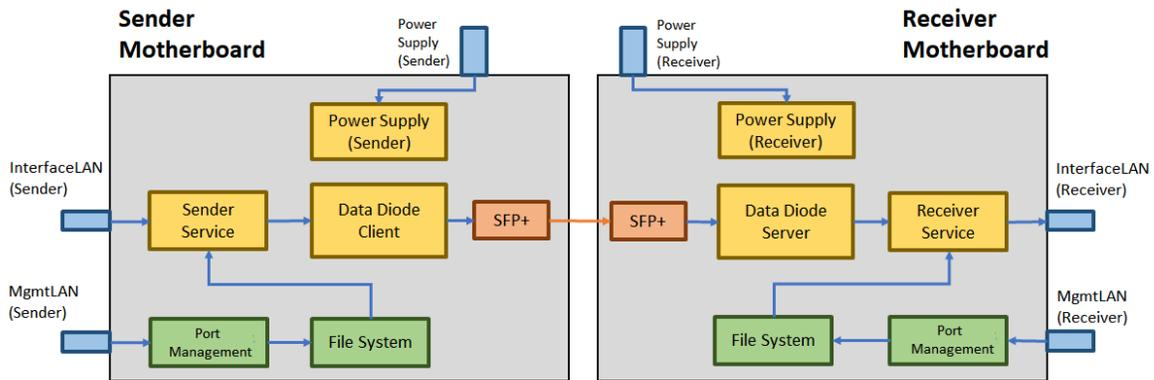
\*Power Supply (Sender) module supplies power to all modules in the Sender Motherboard. Similarly, Power Supply (Receiver) module supplies power to all modules in the Receiver Motherboard. The connections between the Power supply modules and their corresponding modules are omitted in the diagram to keep the diagram readable.
